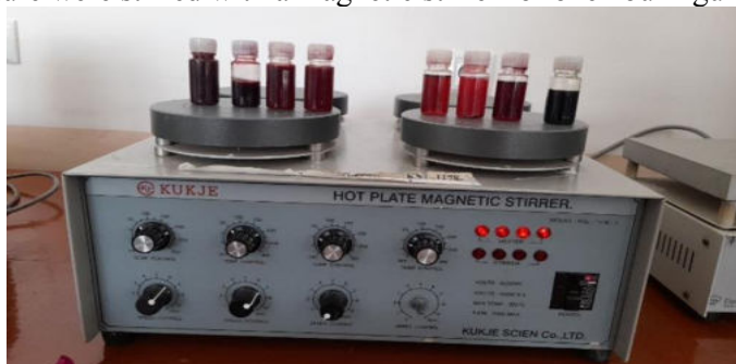
Figure 3 The process of mixing the paint mixture
