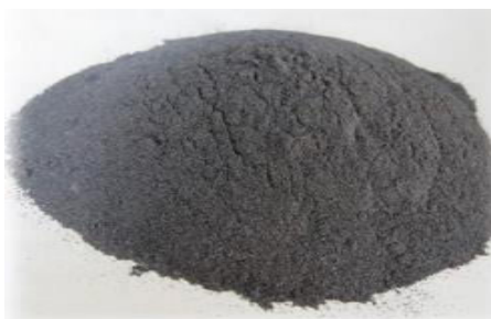
Figure 2. Tungsten carbide powder (20 \mu\text{m} )
