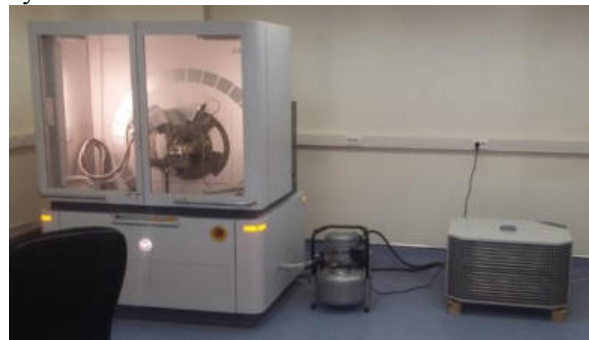
Fig 7. X-ray diffractometer XRD analyzer Empeyan (PANalytical)
