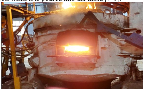
Pic. 2. An electric arc furnace used to liquefy gray cast iron for a lifting roof detail
