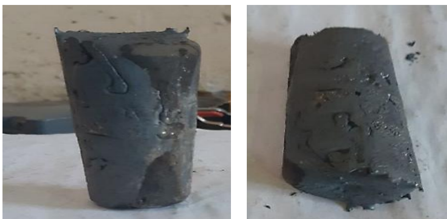
Picture 1. Samples cast in an electric arc furnace from a gray cast iron alloy in a sand-clay mold for research
