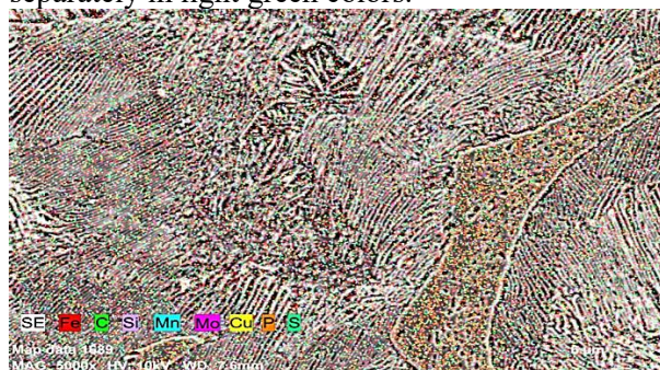
Pic 4: Volume distribution of elements in gray cast iron samples taken by Carl Zeiss Ultra Plus Field Emission scanning electron microscope in the laboratory of the Iron and Steel Institute of Karabuk University
