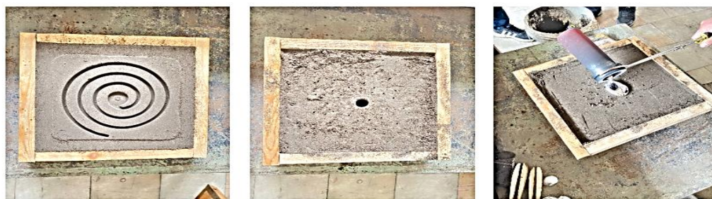
Figure 2. Molds (a, b) and the process of pouring the molten alloy into the mold (c).
