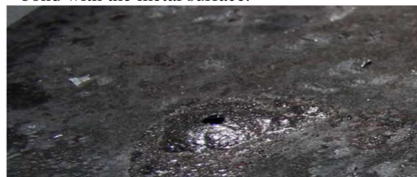
Fig. 2. Surface of the workpiece after hydroscaling: a - with unremoved scale; b - areas of molten scale
