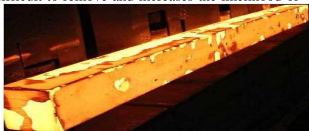
Fig. 2. Surface of the workpiece after hydroscaling: a - with unremoved scale; b - areas of molten scale
