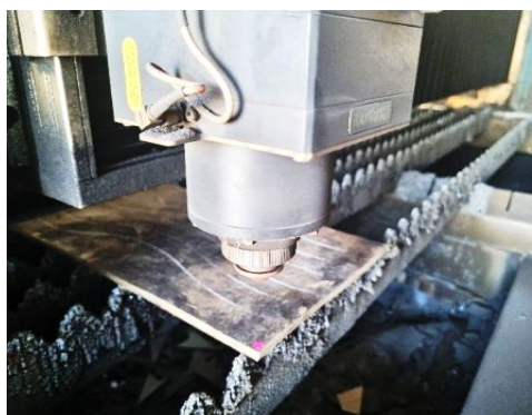
3-rasm. Tanlab olingan 6 mml zanglamaydigan po‘lat materialini lazer mashinasida kesish jarayoni
