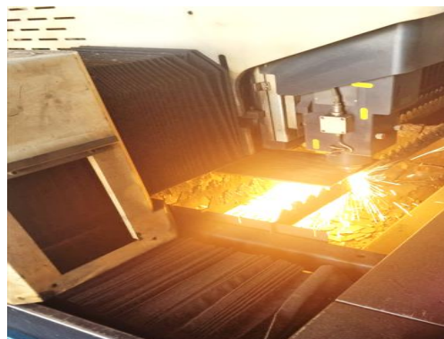
3-rasm. Tanlab olingan 6 mml zanglamaydigan po‘lat materialini lazer mashinasida kesish jarayoni
