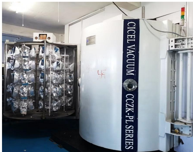
Figure 1. Vacuum installation for obtaining aluminum coatings
