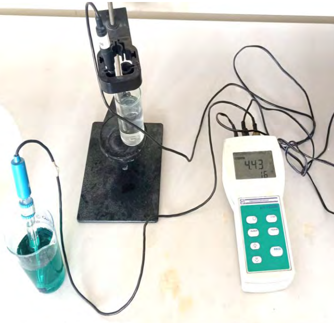
2-rasm. Eritmaga \text{Na}_2\text{CO}_3 aralashtirib cho'kma tushirish jarayoni
